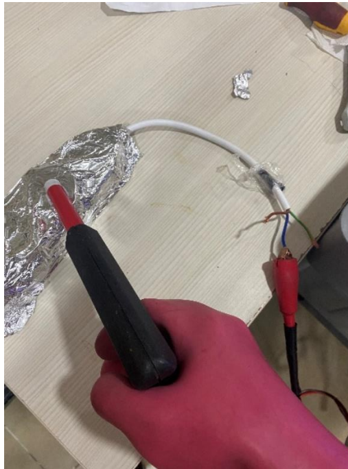
Photo 8. Triple socket-outlet insulation resistance test
