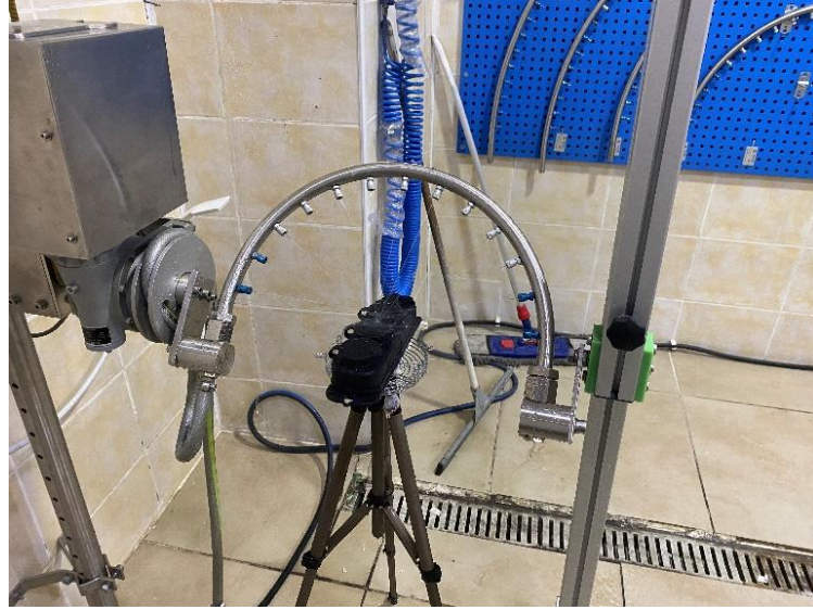
Photo 3. Triple socket-outlet during the test
