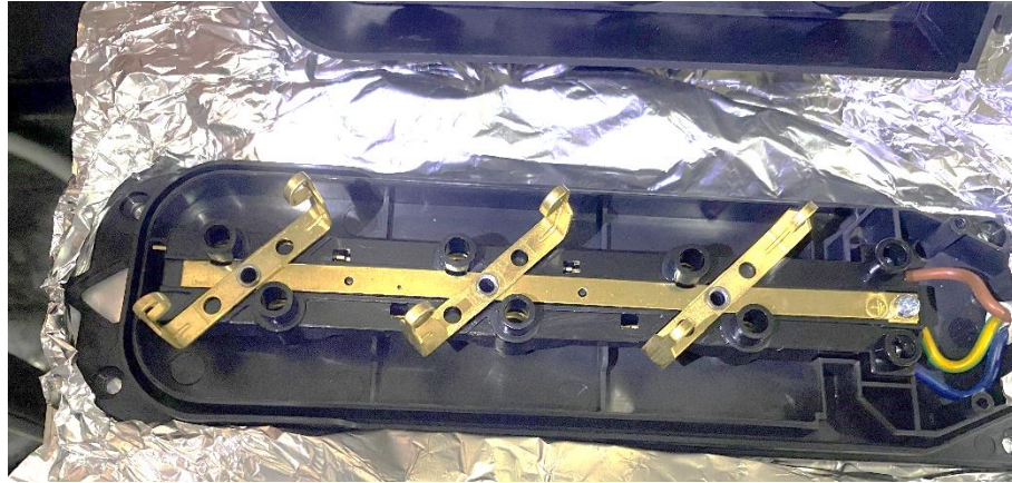
Photo 6. Triple socket-outlet after IPX4 test
