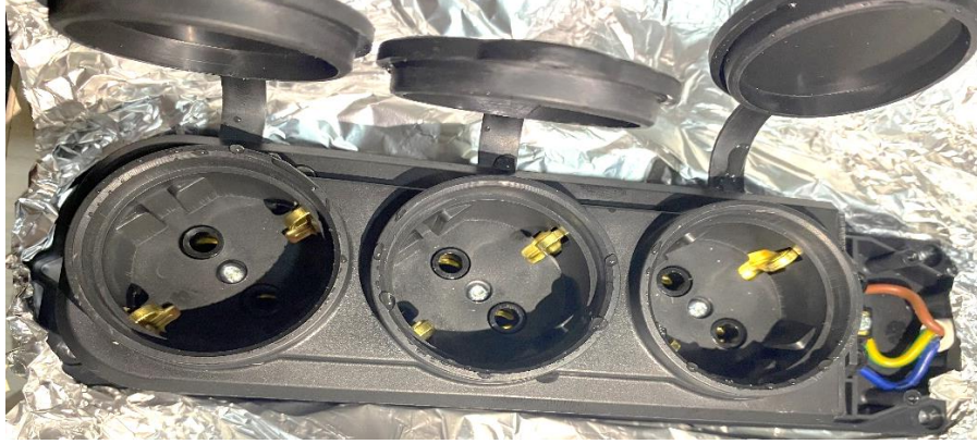
Photo 7. Triple socket-outlet after IPX4 test
