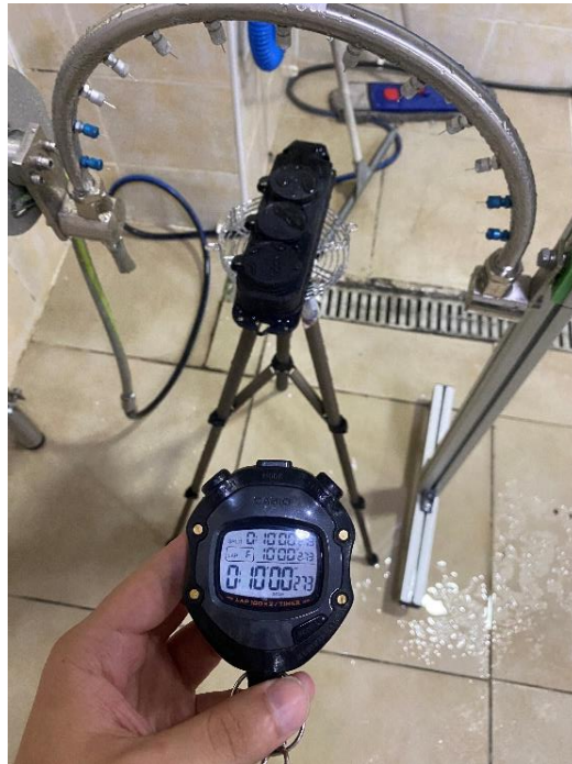
Photo 4. Triple socket-outlet after the test
